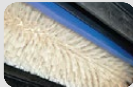
Glycol suction system integrated into sweeping unit
