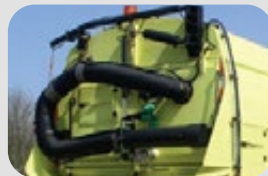
Manual suction system at the rear
